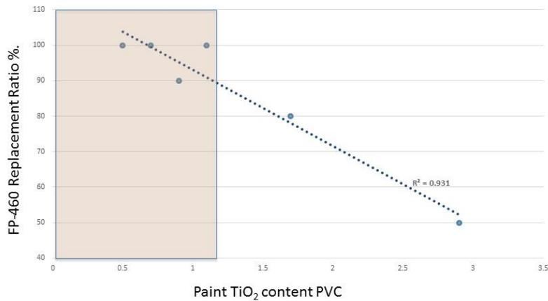
In high PVC paints, at <1% TiO<sub>2</sub> PVC, 100% of the free TiO<sub>2</sub> can be replaced with FP-460.
