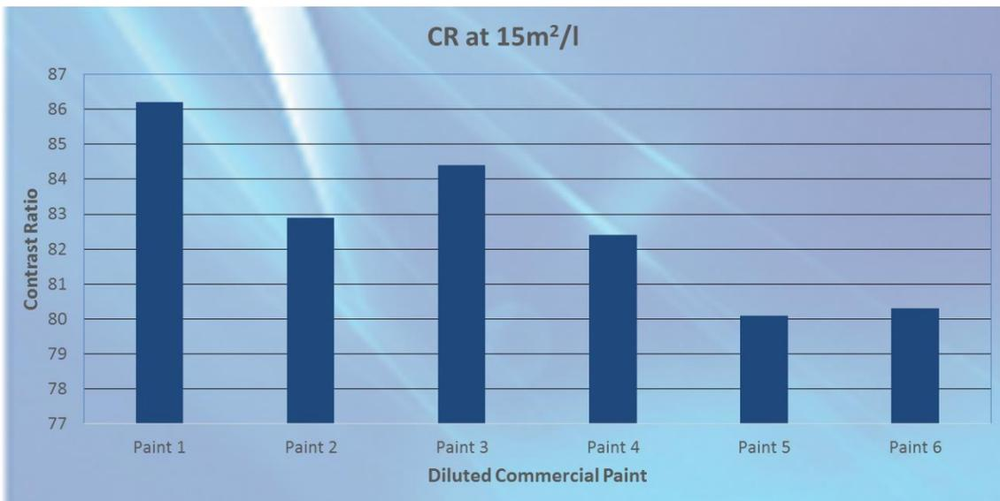
Figure 2: Contrast ratio at a Spreading Rate of 15m<sup>2</sup>/l – all paints diluted as recommended
