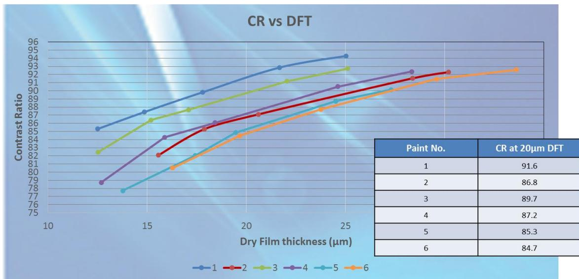
Figure 4. Contrast Ratio vs Dry Film Thickness – all paints diluted as recommended
