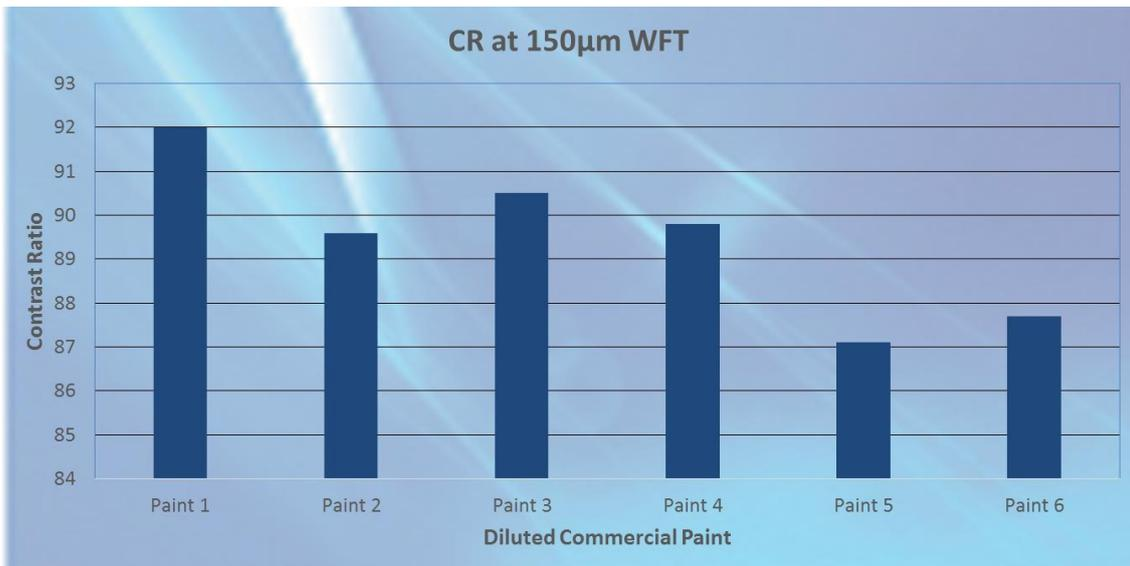
Figure 1: Contrast ratio at 150µm wet film thickness – all paints diluted as recommended
