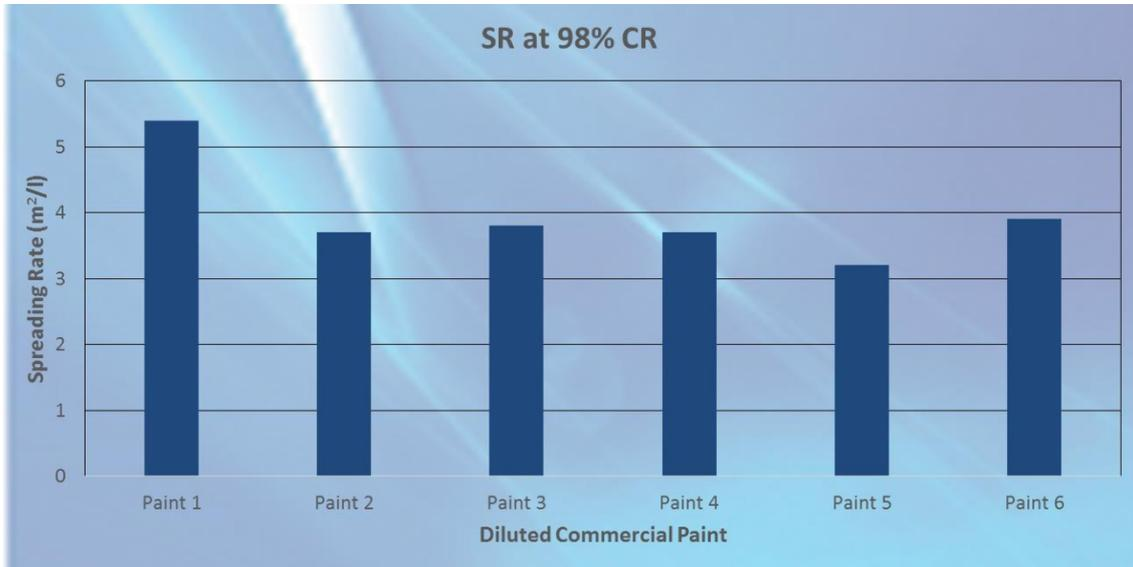
Figure 3: Spreading Rate for a Contrast Ratio of 98% – all paints diluted as recommended
