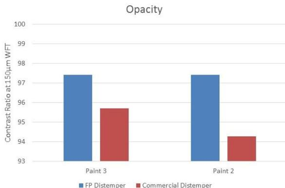
It can be clearly seen that the improved TiO<sub>2</sub> efficiency brought about by FP-Pigments Patented spacing technology provides a boost in opacity compared to the commercial samples and it is this, additional opacity, that allows the formulation to be tailored to local market requirements providing a cost-effective alternative to TiO<sub>2</sub> containing Distempers.
