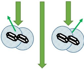
Inefficient scatter as light cannot differentiate between the two particles
