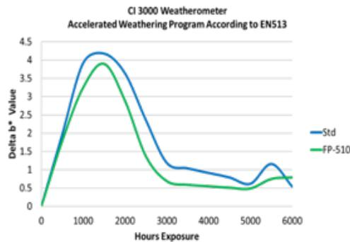
After 6000 hours exposure, the combined colour change for the FP-510 substituted profile is similar to (and perhaps slightly better than) the standard profile. CIE b\* value for the same exposure shows a slight photogreying of the plaque, although this has matched the standard by the 6000 hour mark.
