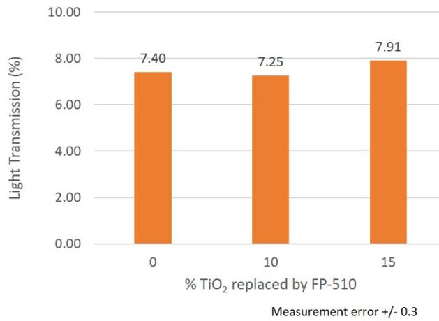
Light transmission behaves similarly at 10% replacement and then begins to rise slightly as more TiO<sub>2</sub> is replaced.
