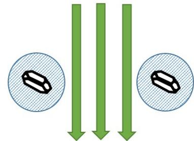
Inefficient scatter as light can pass between the two particles uninfluenced
