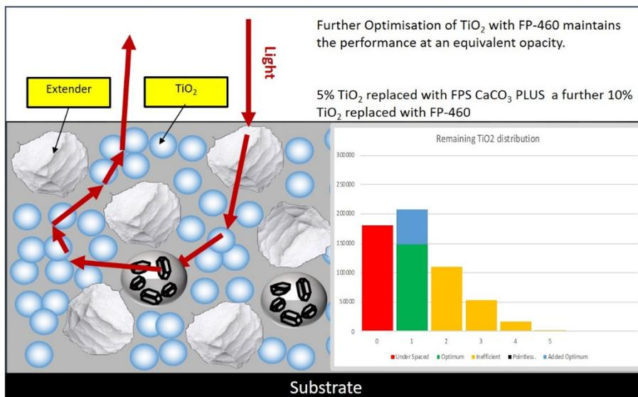
By utilising these performance changes, FP-Opacity Pigments™ can be used in coatings, plastics, inks and paper and board to replace between 5% and 30% of the TiO<sub>2</sub> without significantly reducing the opacity and mechanical properties.
