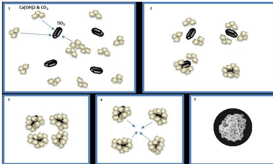
These white pigment composites have an average particle size of 1 micron with a particle of FP-Opacity Pigment™ containing between 3 and 6 TiO<sub>2</sub> particles, each statistically space from each other by the optimum distance for scattering of 280nm.
